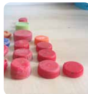
Figure 1: Degradation of caps from highly damaged (far left) to very little damage (far right). Source: The North Sea Foundation, 2017
